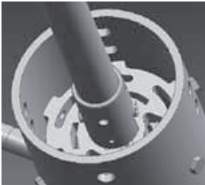
Fig.11 Connection between tap changer body with manual driving mechanism
